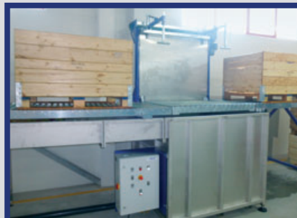
Robotic Bin tipping for two separate infeed flumes
