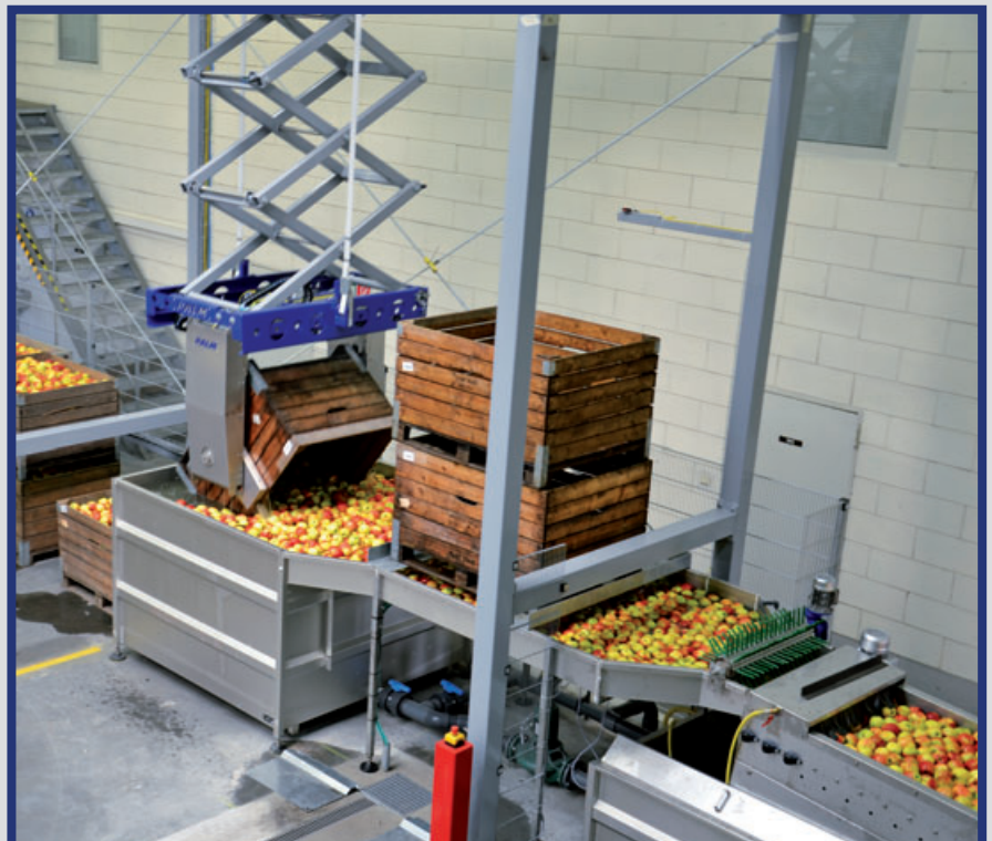
Robotic Bin tipping for two separate infeed flumes
