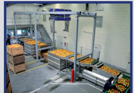
Robotic Bin tipping for two separate infeed flumes
